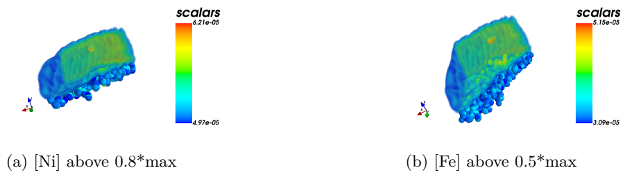
Figure 17: Transition elements with intensities measured above defined thresholds are highlighted within the bulk material
