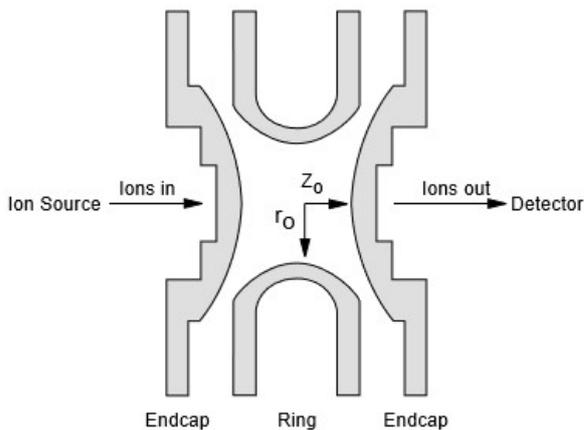
Figure 2: Schematic view of the ion trap
