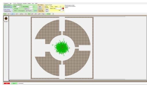
Figure 7: Example using SIMION with asymmetric holes in the ring electrode
