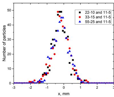
Figure 12: The distribution of the number of particles along the x coordinate (asymmetric geometry)
