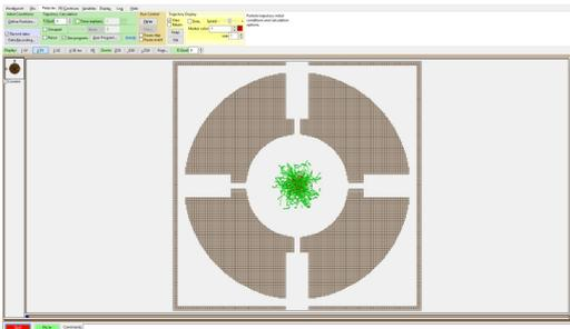
Figure 6: Example using SIMION with symmetric holes in the ring electrode
