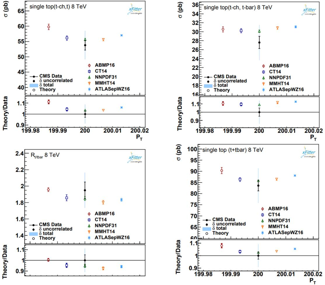
Figure 3: Single top quark and antiquark production cross section predictions, their ratio and the inclusive cross section prediction for different PDF sets (symbols of different style), compared to the CMS measured value [4] at  $\sqrt{s}$  of 8 TeV (filled circle), shown with its statistical (inner error bar) and total (outer error bar) uncertainties.
