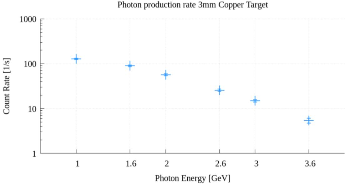
Figure 13: Production rates of photon momenta between 1.4 – 3.6 GeV/c
