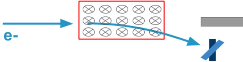
Figure 4: Schematic of measurement setup for deflection position. Electrons travel directly through a magnetic field and to a pair of scintillators.
