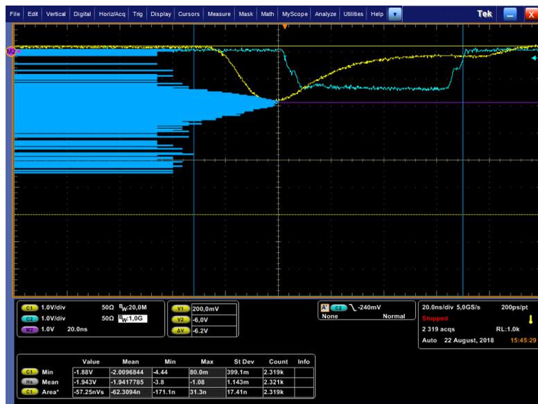
Figure 5: Screenshot from Techtronix MSO500 oscilloscope. The yellow pulse is the signal from the lead-glass detector. The vertical histogram records the pulse minimum value over a period of time
