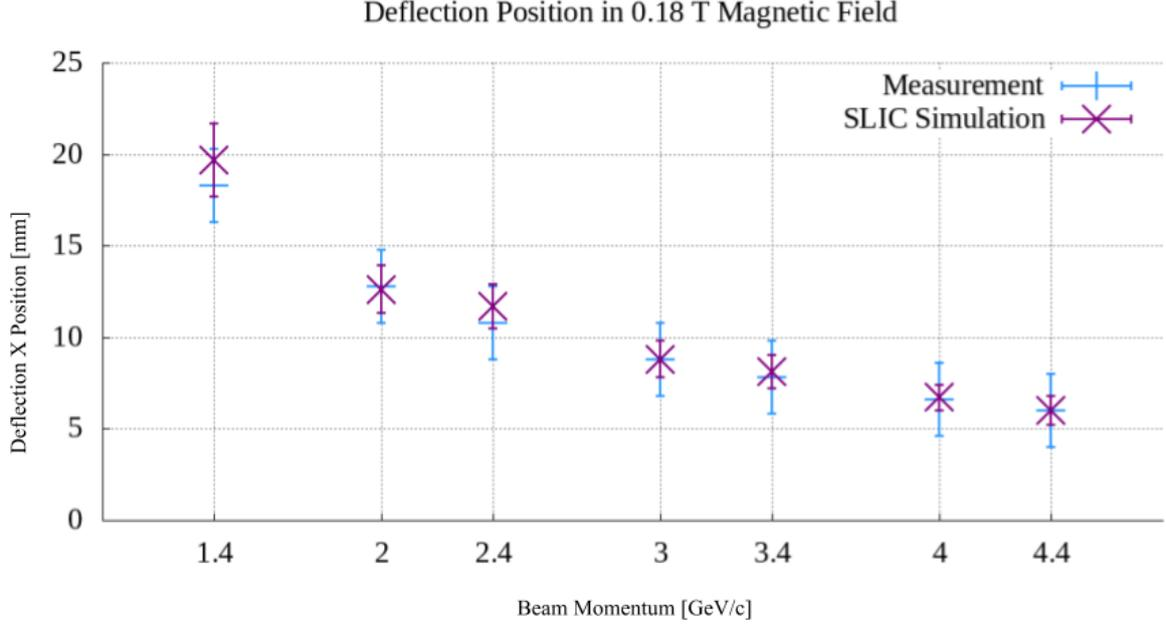
Figure 7: Deflection in horizontal plane of electrons of varying momenta
