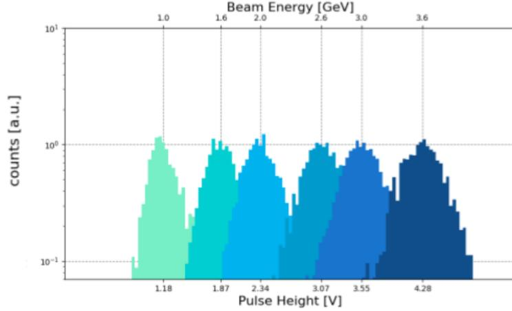
Figure 6: Distribution in Volts of pulse height measured with lead-glass detector.
