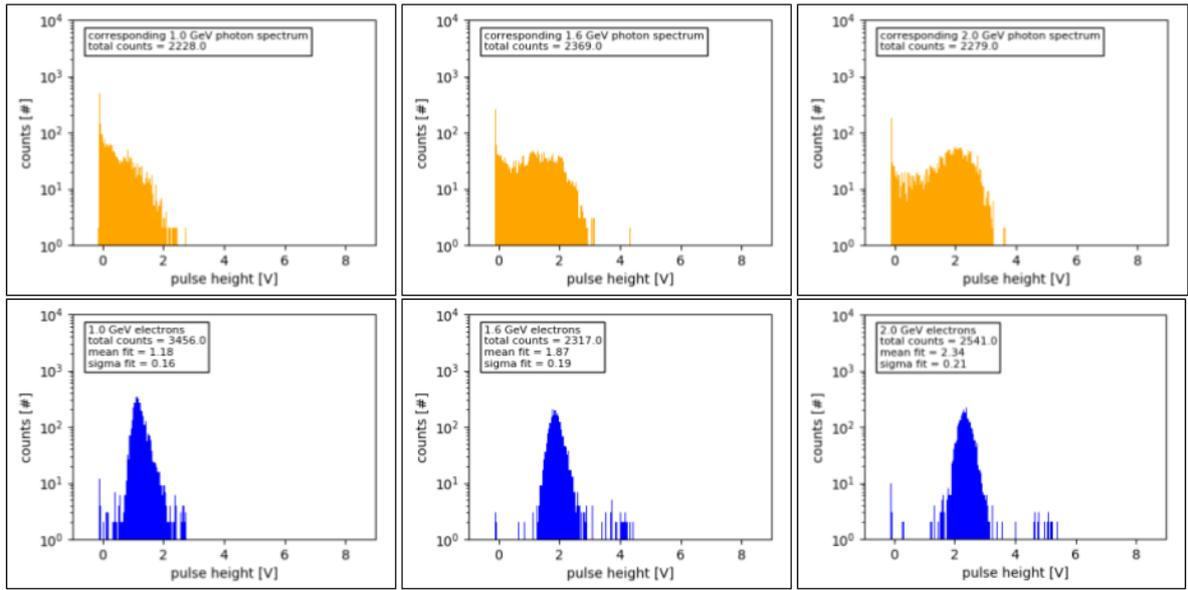
Figure 11: Pulse height distributions of photons in yellow, electron calibration in blue.
