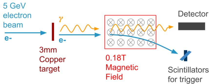
Figure 9: Schematic of measurement setup for photon energy measurements. The measurement in the lead-glass detector is triggered upon a coincidence with the 2 scintillators
