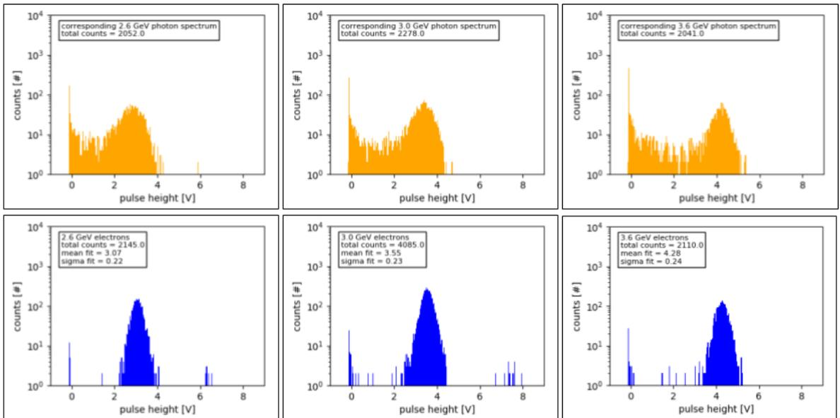
Figure 12: Pulse height distributions of photons in yellow, electron calibration in blue.
