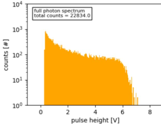
Figure 10: Bremsstrahlung spectrum measured from 5 GeV/c electron beam incident on a 3 mm copper target
