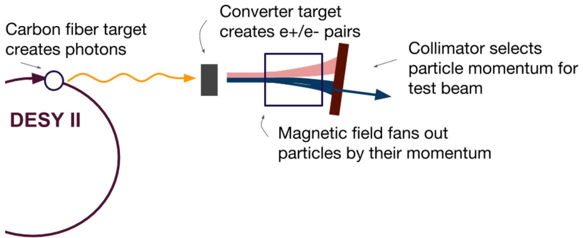
Figure 1: DESY II test beam generation
