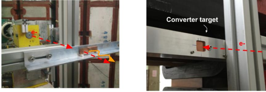
Figure 8: 3mm copper target installed before the magnet. On the left is view towards lead collimator. On the right is view towards magnet
