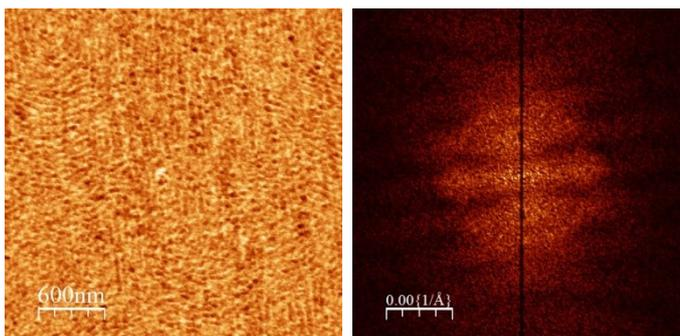
Figure 2: The morphology of samples after solvent annealing with acetone and sputtering with 2 nm of Ag and corresponding images of FFT analysis: (a) presents the sample with heating to 100 °C, (b) presents the sample with heating to 150 °C, (c) presents the sample with heating to 170 °C
