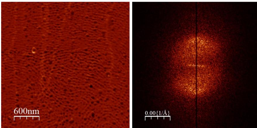
Figure 3: The morphology of samples after solvent annealing with acetone and plasma treatment and corresponding FFT: (a) presents the sample with 5 times treatment , (b) presents the sample with 2 times treatment
