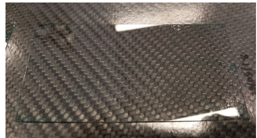
Figure 20: Baseplate and sensor after 24-hour slow glue curing time
