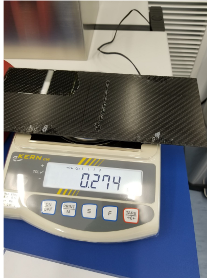
Figure 14: The baseplate was transferred from the rotational stage to the weighing scale to measure the amount of glue
