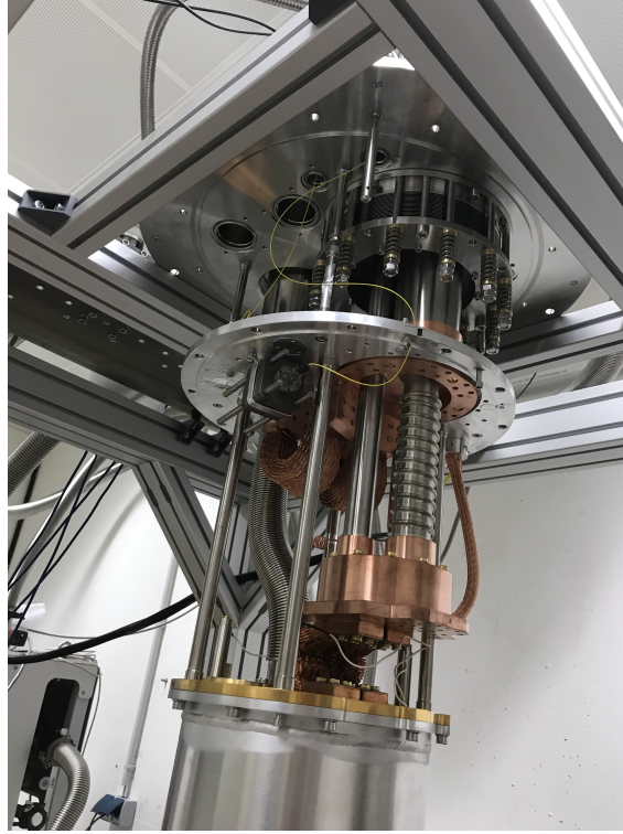
Figure 10: Picture of the filter bench set-up mounted on the lower side of the first flange of the cryostat.
