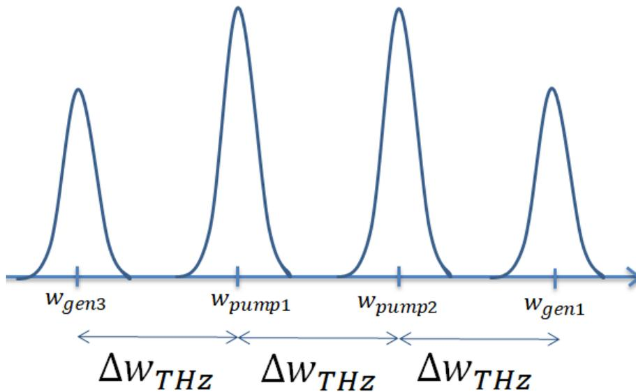
Each couple of the spectral lines will produce two new harmonics and so on. As a result we will have the following situation, that is called cascaded FWM:
