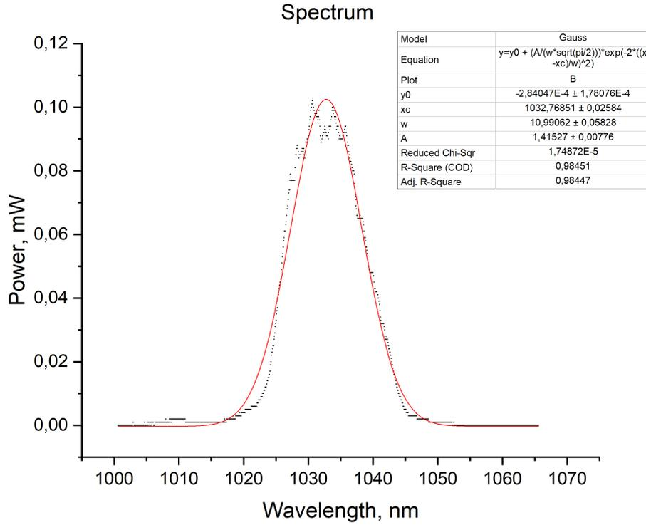
Figure 3: Spectrum of used laser.
