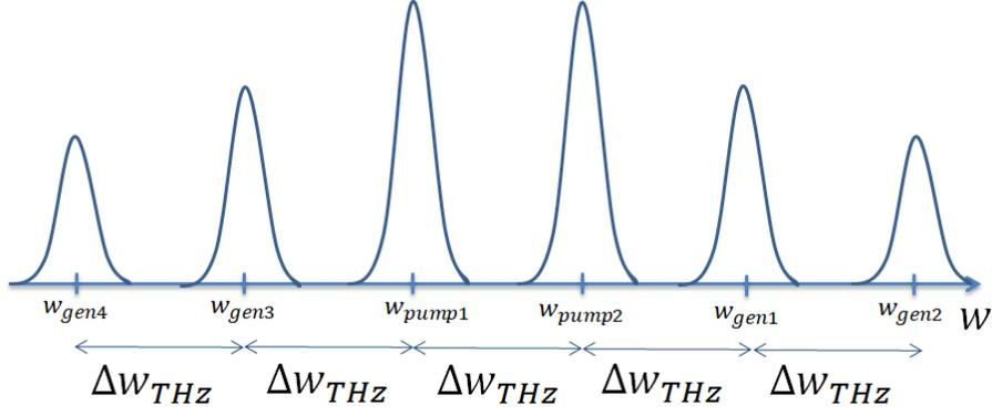
The factor, that limits amount of generated spectral components and determine spacing between them in spectrum, is so-called phase-matching conditions. From mathematical point of view it looks like:
