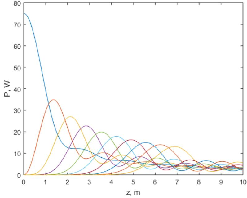
Figure 7: Dependence of power of one pump harmonic and nine generated harmonics on propagation distance in PCF
