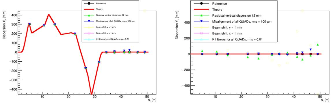
Figure 5: Dispersion in FLASHForward with various effects simulated.
