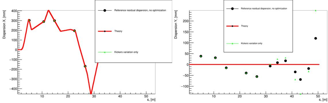
Figure 7: Dispersion in FLASHForward caused by residual disp. with only kickers' parameters variation.
