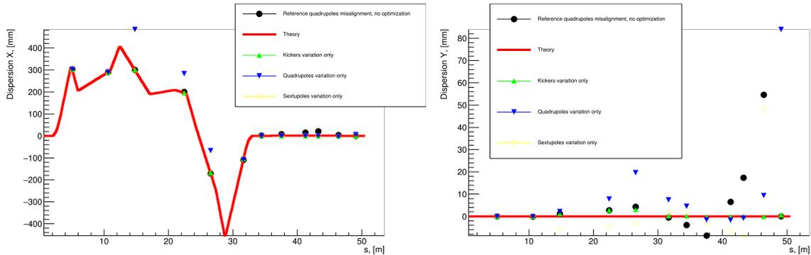
Figure 6: Dispersion in FLASHForward caused by quadrupoles misalignment with different optimization approaches.
