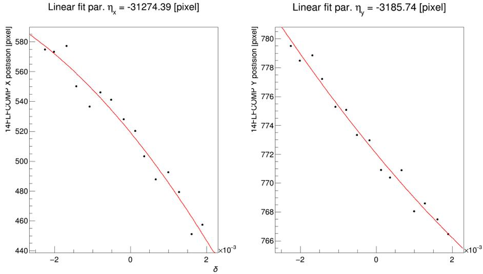
Figure 8: Dispersion at 14FLFCOMP calculated using screen data.
