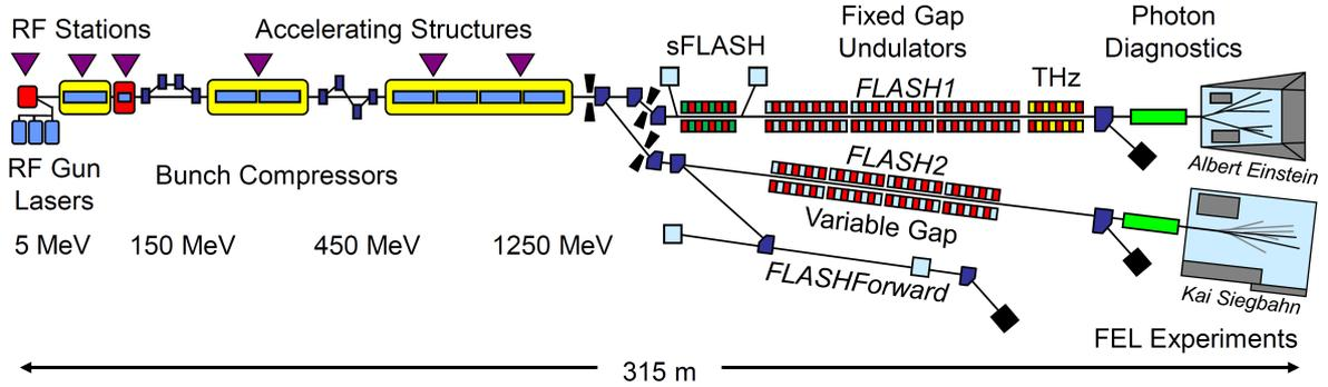
Figure 1: Schematic layout of FLASH. Not to scale.
