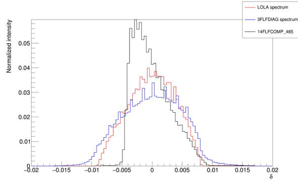
Figure 9: Beam energy distribution obtained in 14FLFCOMP, 3FLFDIAG and LOLA.
