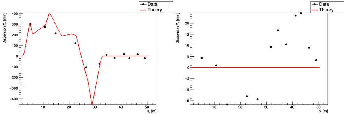
Figure 4: Measured horizontal and vertical dispersion distribution along the FLASHForward beamline.
