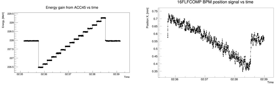
Figure 2: Energy gain of ACC45 and beam horizontal position in 16FLFCOMP BPM recorded by the DAQ system.
