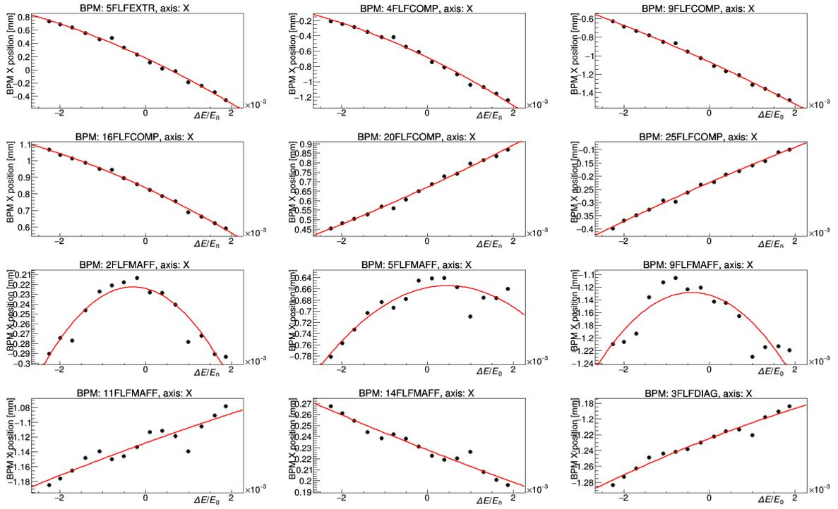
Figure 3: Beam horizontal position as a function of energy gain for all BPMs in FLASH-Forward.
