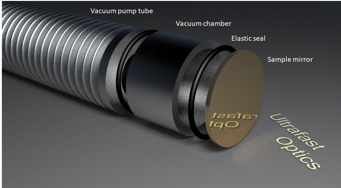
Figure 1: Simplified illustration of tunable-focus high-reflector.
