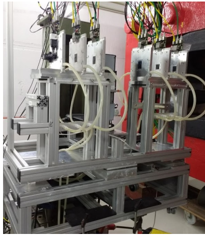
Figure 1: The DURANTA beam telescope
