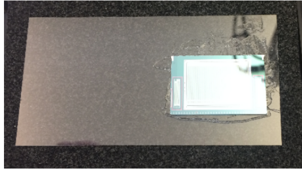
Figure 13: Silicon piece mounted on glass plate
