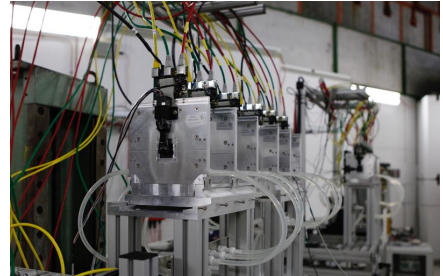
Figure 5: Telescope at the DESY test beam facility
