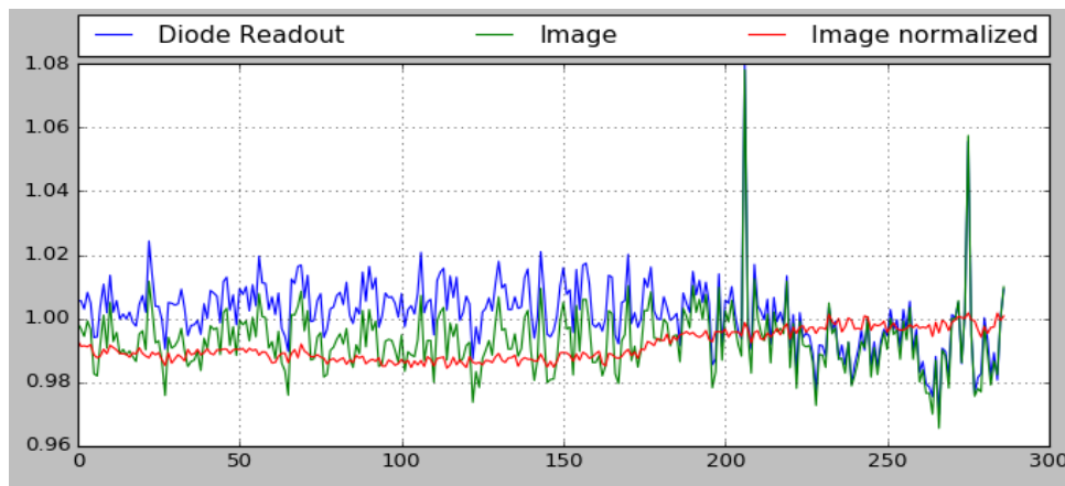
Fig.9 Line plot (marked in red in Figs. 7,8,10) through the diode readout, raw image and normalized image.
