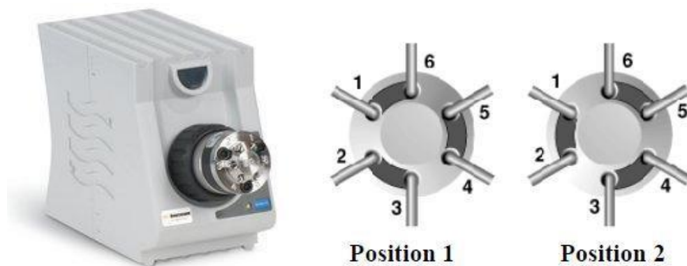
Figure 4. Scheme of switching valve positions.
