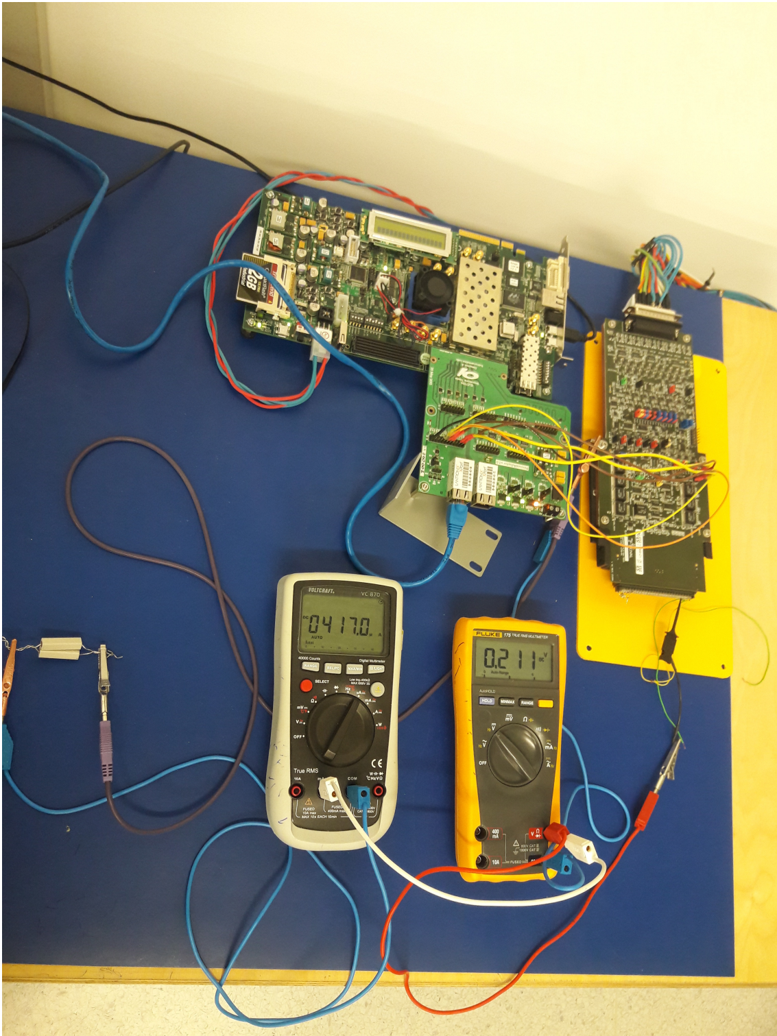
Figure 4: Current monitoring setup.
