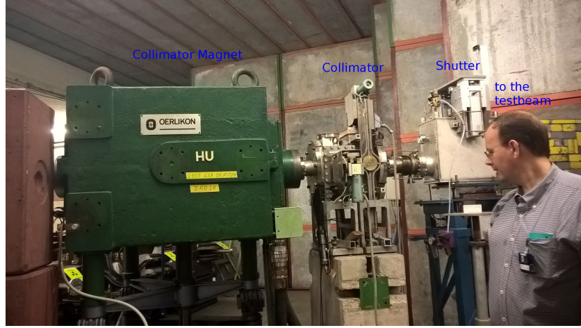
Figure 4: A foto of the setup for test beam production with the DESY test beam coordinator Marcel Stanitzki on the right side
