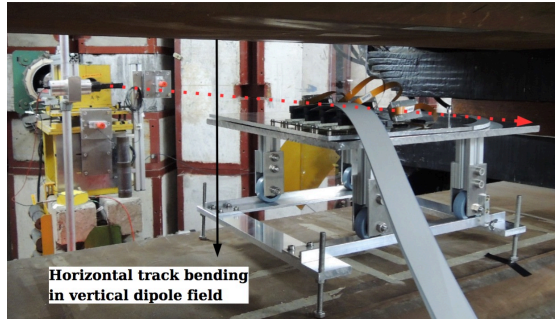
Figure 5: Four CMS silicon pixel modules mounted on a rotatable plate inside the homogeneous field of a dipole magnet. The incident electrons are indicated by the dashed red line, and the direction of the dipole field lines by the black arrow. The electrons are bent in the horizontal plane due to the Lorentz force (Sec. 3.1).
