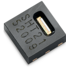
(a) Sensor SHT21 (Humidity & Temperature). 6 GPIO pins connections.
