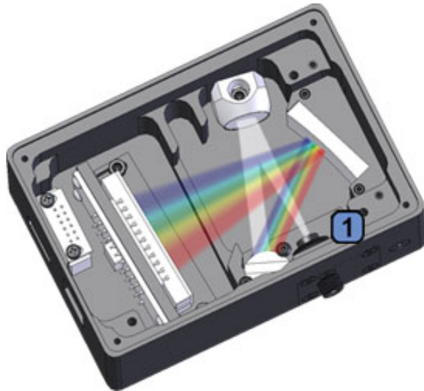
Figure 2: Example of the inside of a typical spectrometer. Light enters at the point labelled 1 and follows the path shown, onto a mirror and diffraction grating before being reflected onto the detector. (BW Tek, 2016)
