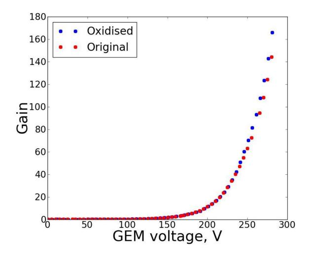
As we can see, gain does conserves in GEM after oxidation procedure. This opens us new perspectives to use this oxidation technology to increase GEM stability against discharges.
