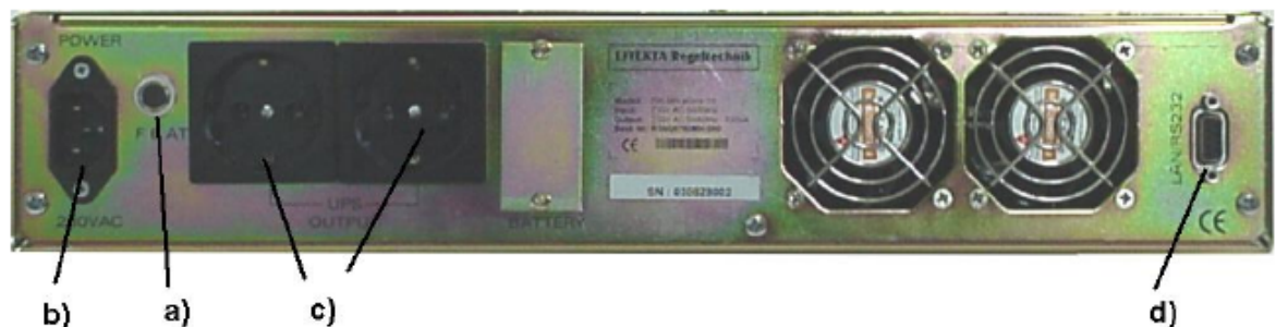
Figure 4.7: The rear panel view of the UPS a) Fuse at mains power input, b) Mains power c) UPS output d) Communication
