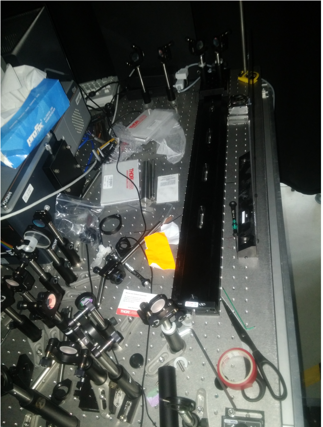
Figure 12: Delay line and FDI beam path
