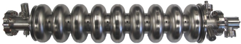
Figure 1: Picture of Tesla-shape nine-cell SRF niobium cavity
