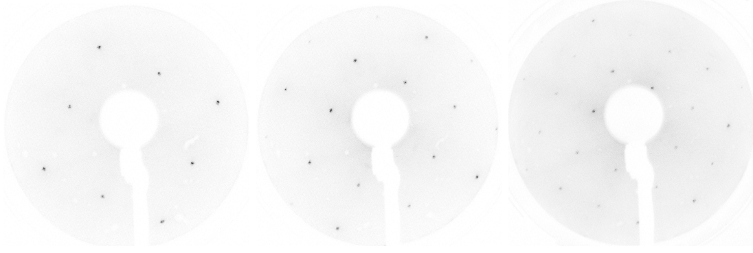
Figure 7: Color inverted LEED patterns of the bare STO at 70eV (left), 100eV (middle) and 170eV (right).
