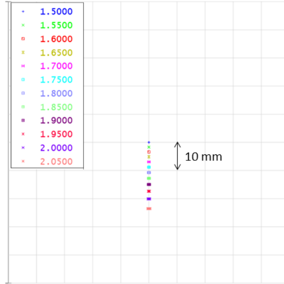
Figure 15: Spot diagram at the detector position for G1 setup
