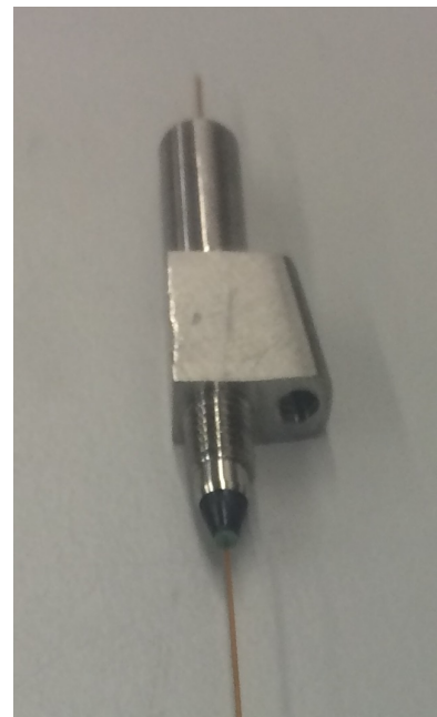
(c) A.3) metal ferrule is slipped on from the back of the capillary.
