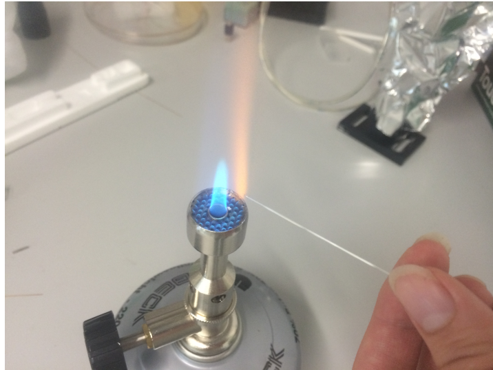
Figure 2: Melt the outer glass capillary in a bunsen burner flame while rotating it. Have a look in the microscope and try to fit a grinded inner capillary. Iterate until satisfactory protrusion length ( 200\text{ }\mu\text{m} to 350\text{ }\mu\text{m} ).
