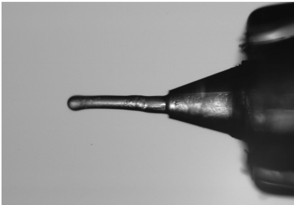
Figure 14: Testing with lysozyme crystals did not give a stable jet. Flows with different speed was observed within nozzle.
