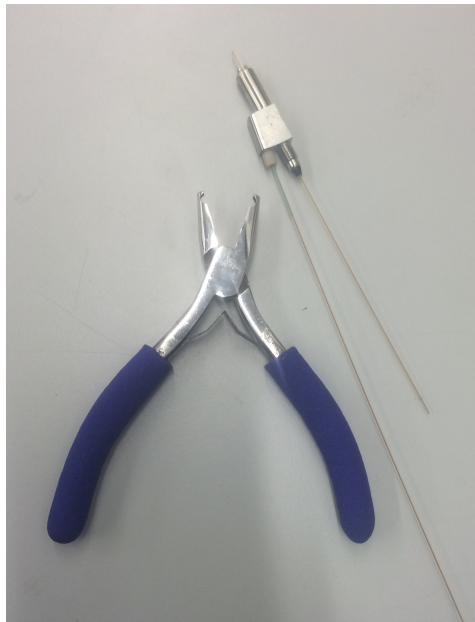
Figure 9: A fully assembled nozzle body shown with the special pliers for tightening the gas line.
