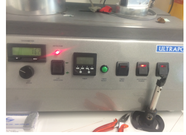
(c) The rotating motor is set to 3000 rpm. Accessory power is turned on and the lap direction set to (-).
