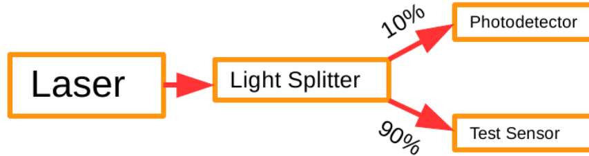
Figure 4: Schematic view of the light splitter.
