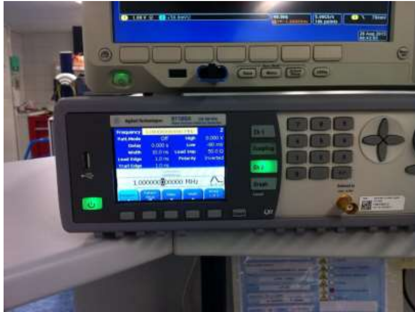
Figure 12. Pulse Generator configuration
