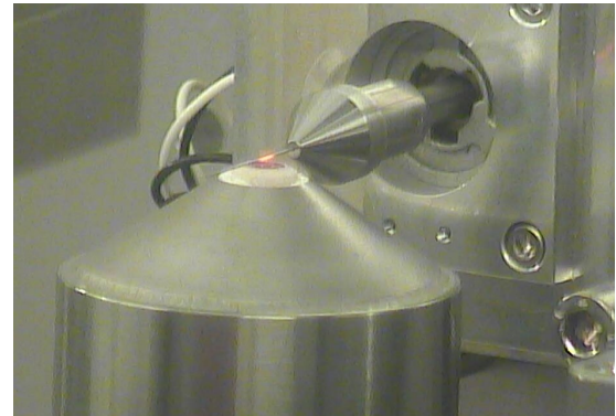
Figure 4: Silicon calibrant in a spinning capillary during the experiment, T_{HAB} = 1000^\circ\text{C}
