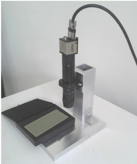
Figure 9: Camera holder with camera and PS module
