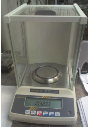
Figure 1: Weighting elements on a digital scale with a 10^{-3} precision.
