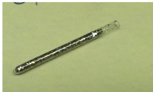
Figure 9: Quartz capillary filled with milled metallic glass ribbon.
