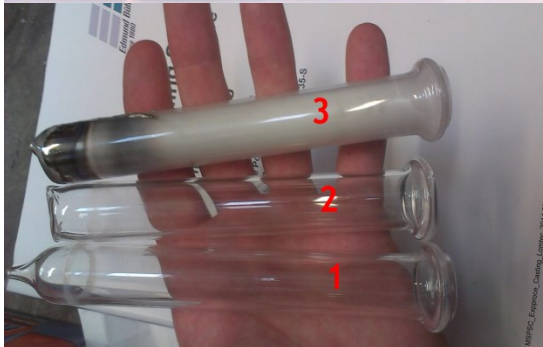
Figure 6: Quartz nozzles: before use with cylindrical shape ending (1), before use with rectangular shape ending (2), after use with rectangular shape ending and coated inner surface with BN (3).
