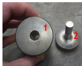
Figure 2: Ramming in the die ((1) body of die, (2) moving part) by using mechanical press (3) with maximum power 98000 N.
