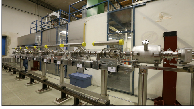
Figure 5: E-XFEL 3rd harmonic accelerating module
