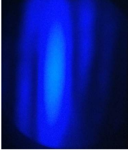
Figure 29: Fluorescence of 256nm harmonic from the white paper. The shot of the part of the beam is taken by external camera at some angle
