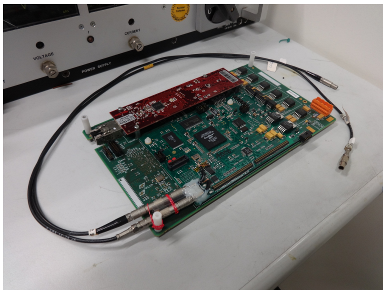
Figure A.13: The Readout Control Unit (RCU).
