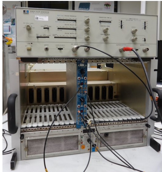
Figure A.24: In the top the pulse generator we used to create a pulse can be seen. Visible at the bottom is the dual gate used by us as trigger for trigger box and pulse generator. Also, one can see the NIM rack and power supply used.
