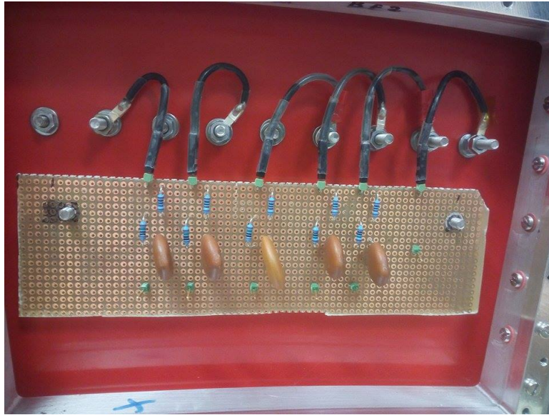
Figure A.8: The module board installed on the module. Visible are also the screws that made the module gas tight. The big capacitor in the middle had 5 kV voltage resistance and was planned to be used for the COM. All others had 2 kV voltage resistance. On the right one can see the connection to the copper plate. Courtesy of Oleksiy Fedorchuk.
