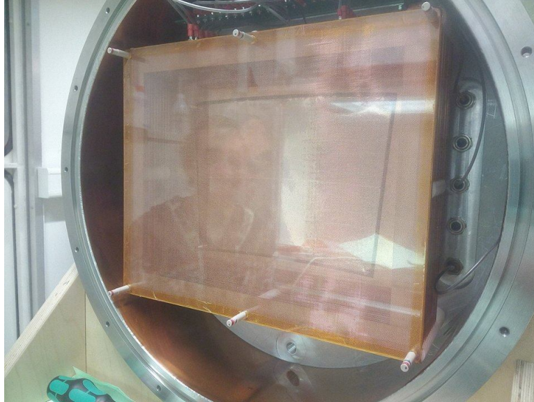
Figure A.10: The cathode, anode, field formers and a GEM are visible. At the top, one can also see parts of the field board.
