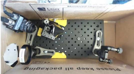
a) **Fig 6.** a) The real set-up b) The knife-edge detection unit
