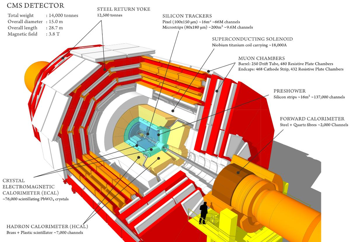
Figure 5: Sectional view of the CMS detector
