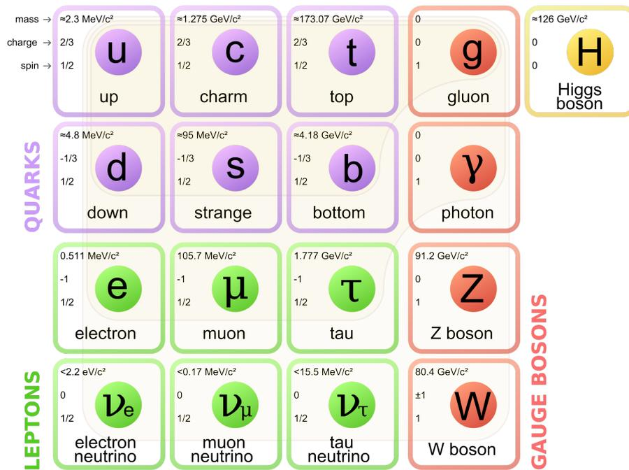
Figure 1: The SM elementary particles together with their mass, charge and spin[1]
