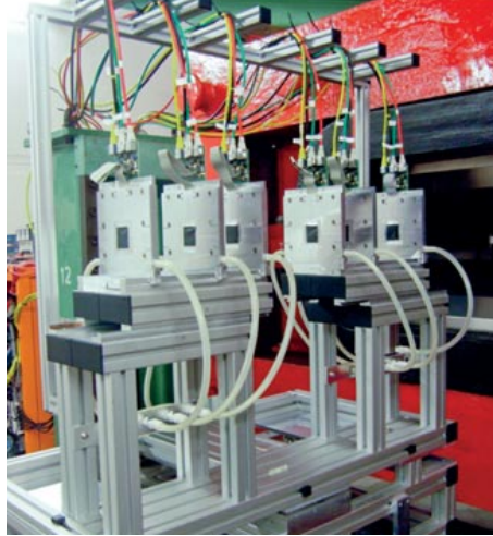
Figure 2: The sensor telescope used with the 5 GeV DESY testbeam. This telescope is based on the EUDET telescope and is called the Datura pixel telescope. The device under test is placed at the centre of the system, with three sensor planes either side. Each plane contains a Mimosa 26 sensor, which is used to record the particle hit data.
