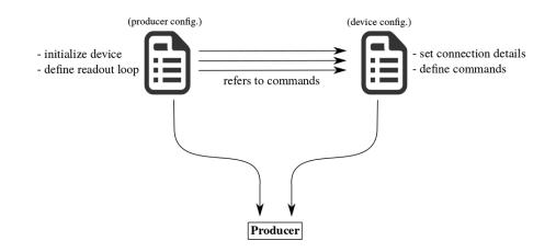
Figure 2: Construction of a generic producer by configuration files. The fact, that one producer configuration can refer to multiple device configuration files is not shown.
