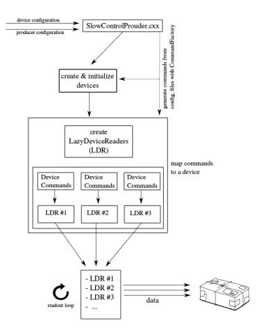
Figure 3: Work flow of a Slow Control Producer
