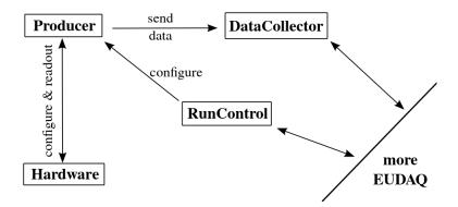
Figure 1: Relevant parts of the EUDAQ-framework architecture.
