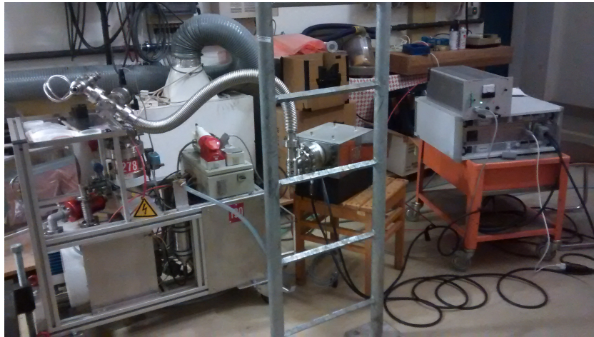
Figure 21: The set up of the NEG/Ion pump and turbo-molecular pump station(from left to right).
