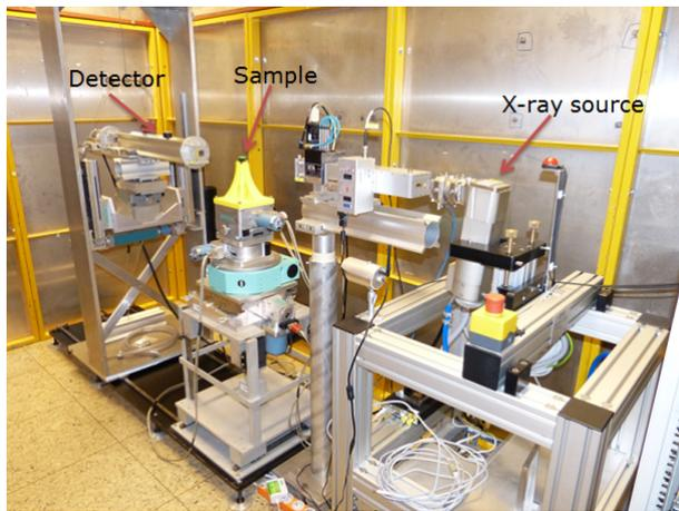
Figure 9: X-ray reflectivity setup
