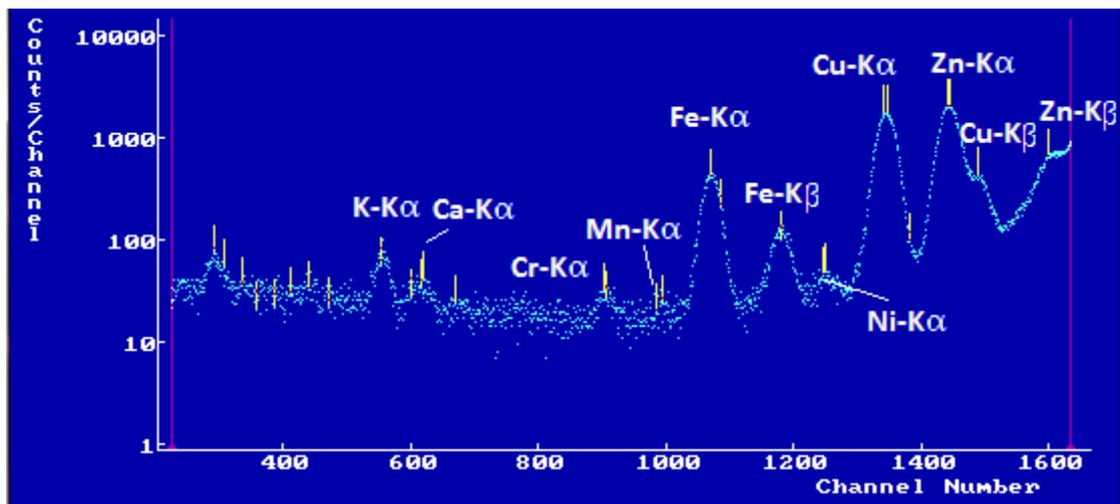
Fig. 4. The XRF spectrum of the examined sample.
