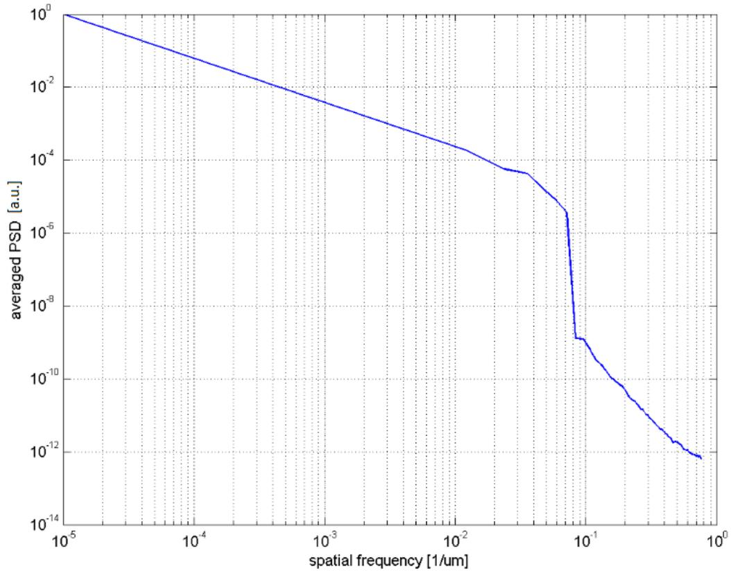
Fig. 5. Averaged power spectral density values in the function of spatial frequency for transmission data. The boundary frequency is  $0.3/\mu\text{m}$ . It corresponds to the resolution of  $1.67 \mu\text{m}$ .
