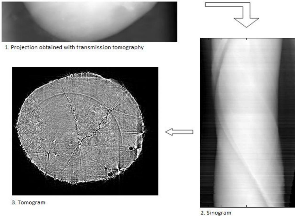
Fig. 2. Picture 1 represents a projection collected by transmission detector. Picture 2 illustrates a sinogram, which lets us make a tomogram (picture 3). For this inverted Radon transform was utilized.
