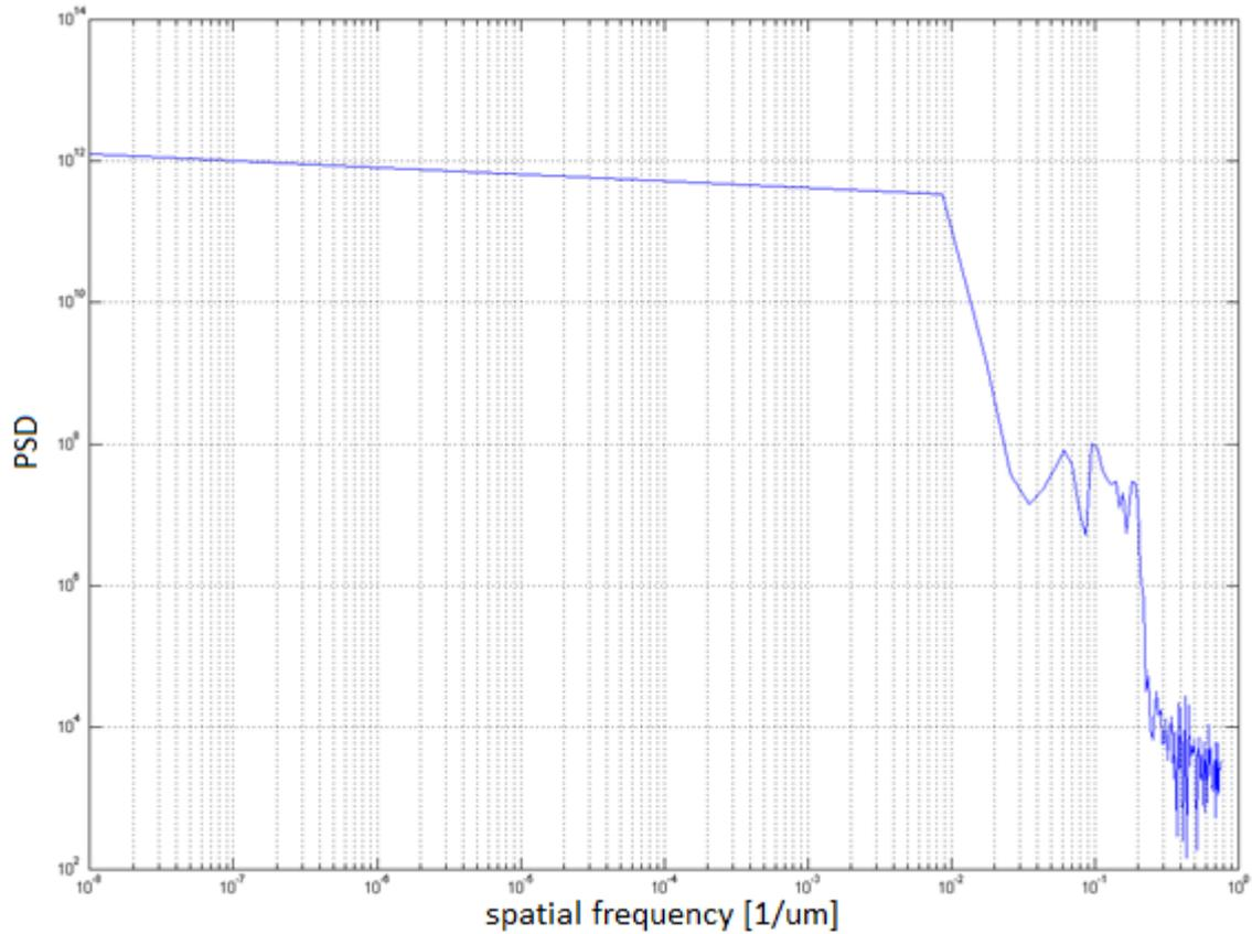
Fig. 8. Power spectral density values in the function of spatial frequency for transmission data. The boundary frequency is 0.4/um. It corresponds to the resolution of 1.25 um.
