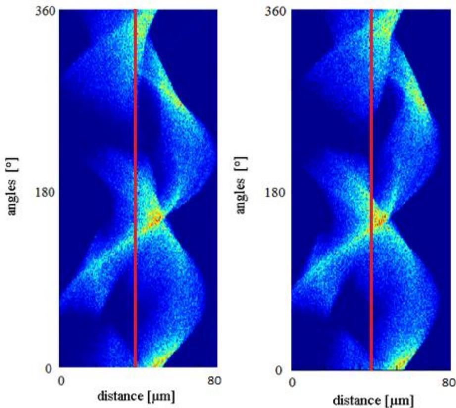
Fig.3. Sinograms of calcium  $K\alpha$  line; uncorrected sinogram is on the right, corrected on the left. The red lines represent rotation axis of the sample.
