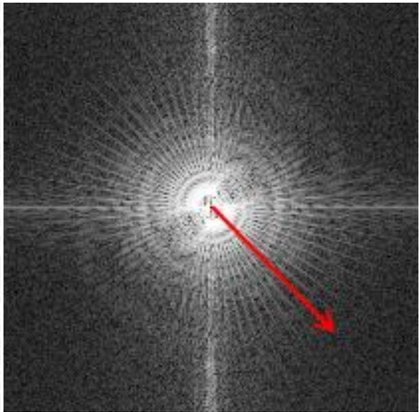
Fig. 7. Power spectrum of an image. Values of pixels under the red line are taken into account when preparing PSD in the function of spatial frequency - chart (Fig. 8).
