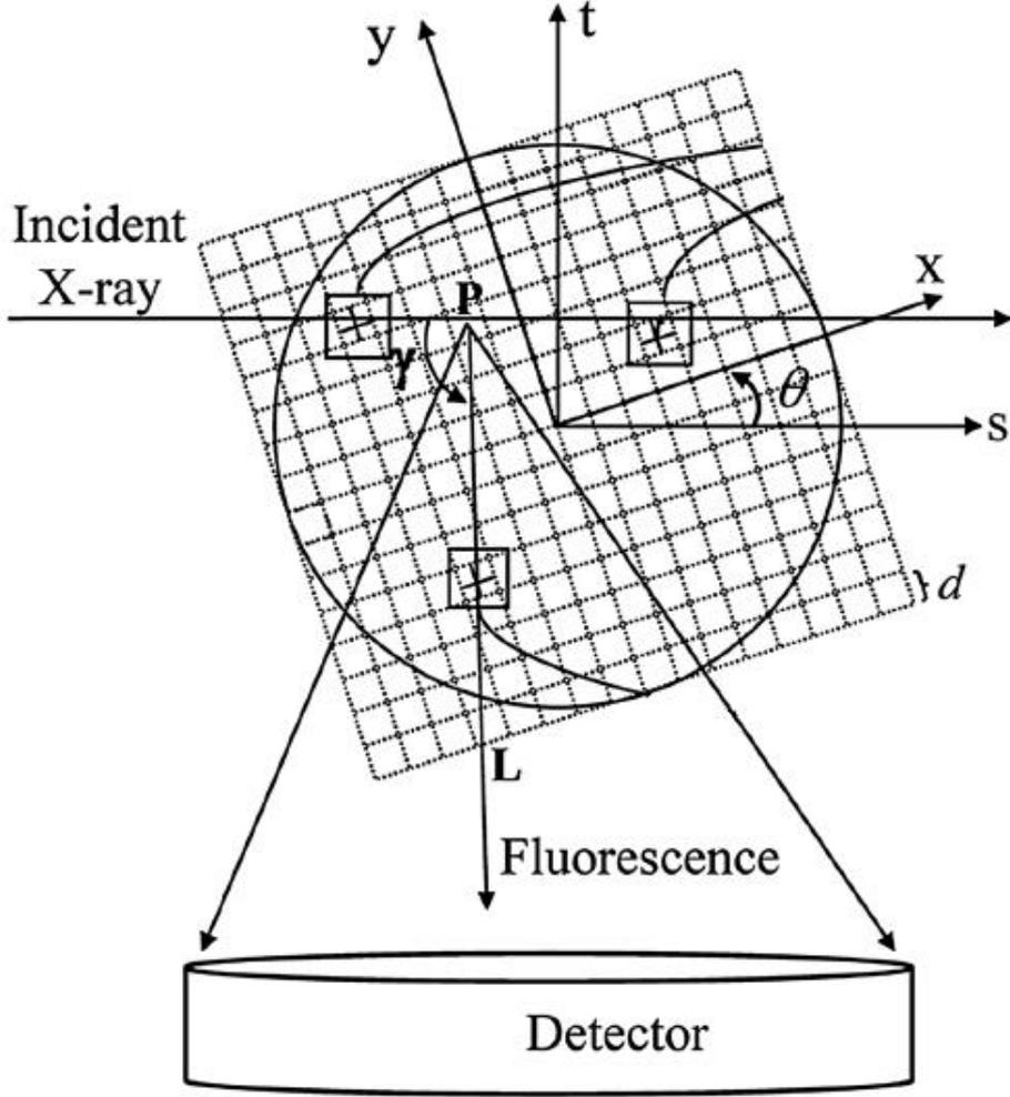
Fig. 10. Schematic diagram of the acquisition geometry of XFCT, where  $xy$ -coordinate and  $st$ -coordinate systems are fixed to the object and the laboratory, respectively.  $d$  is the size of the pixel.  $L$  denotes the distance from point  $P$  to the edge of the object.<sup>ii</sup>
