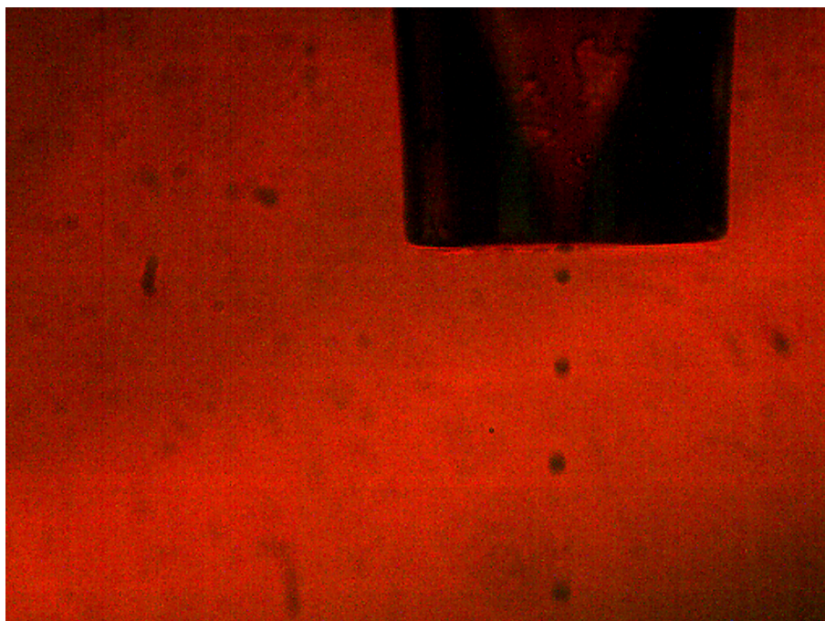
Figure 2: Water droplets ejected from the nozzle with a strobe delay of 125 \mu s.
