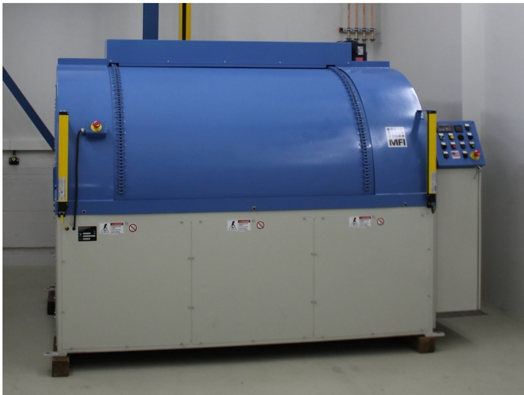
Fig 15: Centrifuge used to polish cavities at HiGrade HiGrade laboratory.
