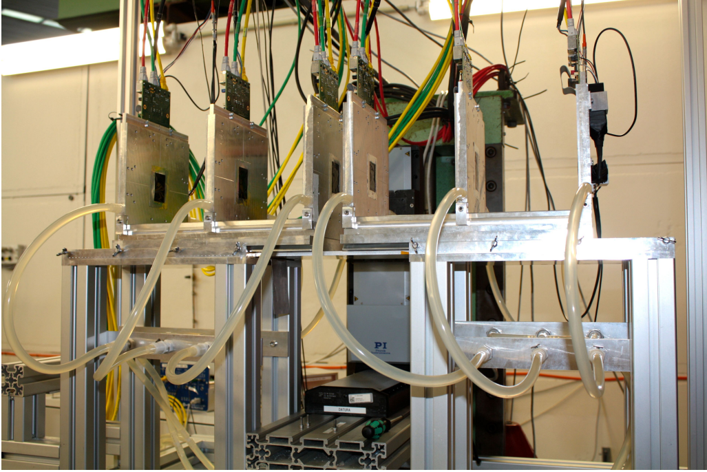
Figure 2: The DATURA beam telescope. The MIMOSA26 pixel sensors and their readout systems are mounted on aluminum planes. The arms of the telescope can be moved apart in order to place a DUT (Device Under Test), such as a pixel detector prototype, in the middle of the telescope. In front of the first plane (right) and behind the last plane (hidden in this perspective) two crossed scintillators each are located, which are used for a fourfold coincidence trigger. Beam incident from the right. The assembly had to be changed for the experiment in this project in order to get tracks with hits in every sensor plane. Figure 5 shows the actual experimental setup. [3]
