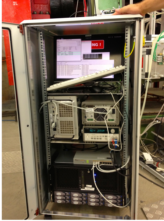
Figure 3: Data acquisition system for the DATURA beam telescope, consisting of (from the bottom) a RAID storage, the RunControl PC, a LAN router, two power supplies and a National Instruments PC, mounted into a 19" rack. The Trigger Logic Unit and the JTAG and Clock distribution boards are hidden on this image.
