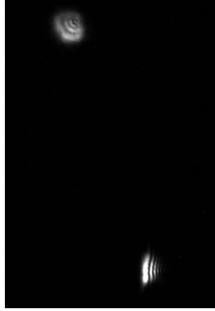
Figure 6: Two spots can be visible with alignment laser.
