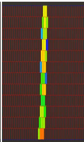
Figure 5.2: Pulses over the pads (200 \mu\text{m} diffusion).
