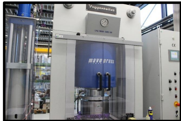
Fig 1 . 100ton Large Volume Press at HASYLAB DESY, Hamburg .
