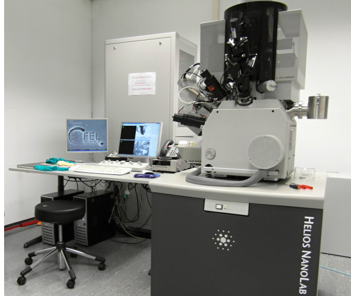
Figure 3: The dual beam system combines functions of scanning electron microscope and focused ion beam
