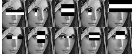
Figure 13: Haar-like features used to detect a human face.
